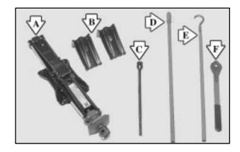
The tools you'll be using include the jack (A), the wheel blocks (B), the wheel wrench (C) jack handle extension (D), the jack handle (E) and the ratchet (F).
